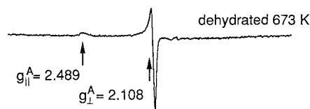
Figure 12. ESR spectrum at 77 K of isolated Ni(I) in NiH-SAPO-11.
